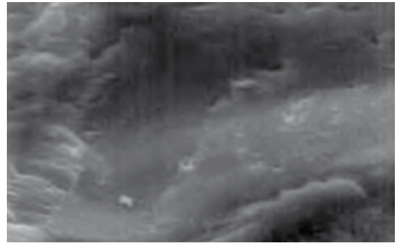
Cement with NovoCrete®: closed dense structure
