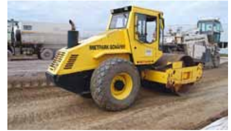
Static and dynamic compaction
